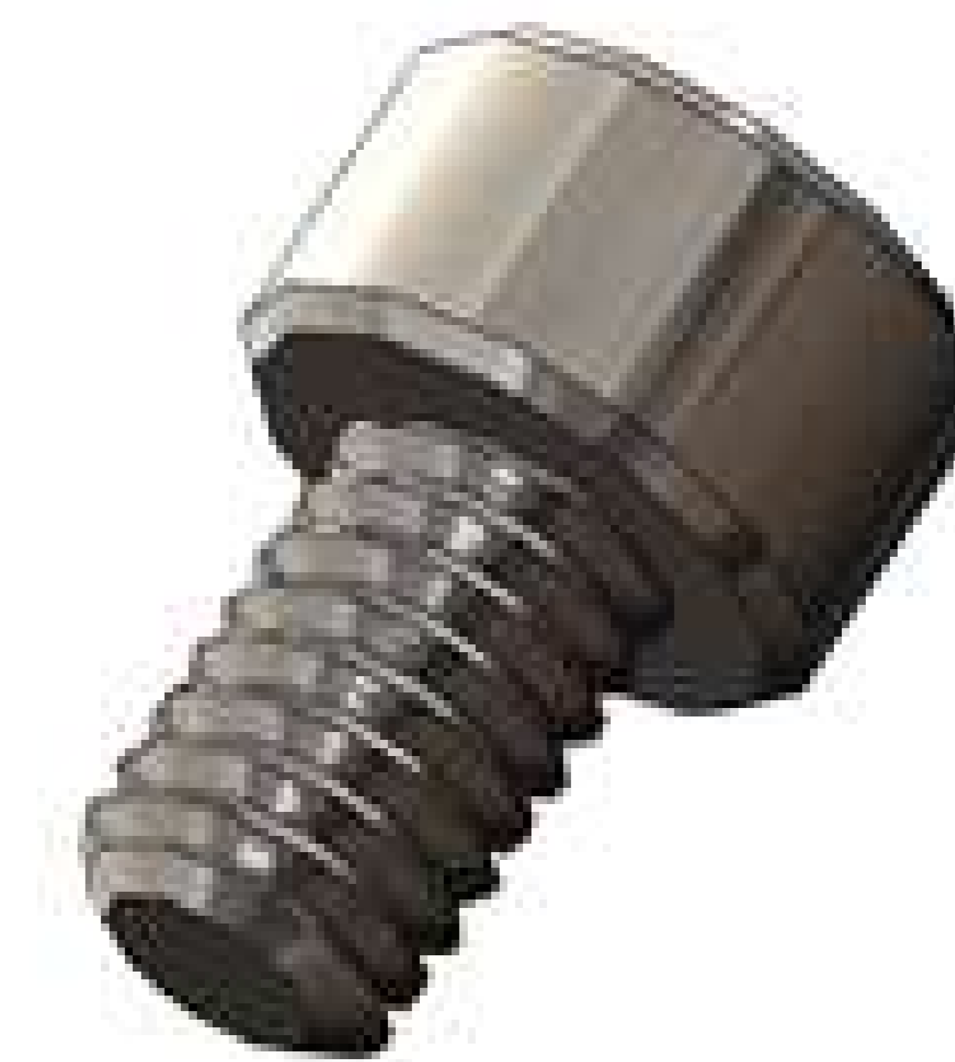
3. Screw CHC ISO4762-M04X006-A4-70 ST316SCHM0406
